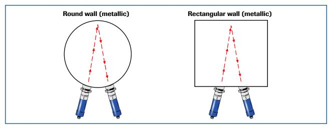
Fig. 2: Installation on one site of pipe
