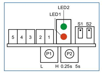
Fig. 3: Electrical connection receiver
